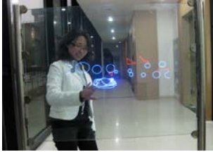
Sample image projected on film with dual color projector. Images move and flip, like a hologram that can be read on both sides of the window.
