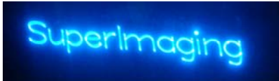
Sample image projected on film. Images move and flip, so messaging looks like a hologram and can be read on both sides of the window.
