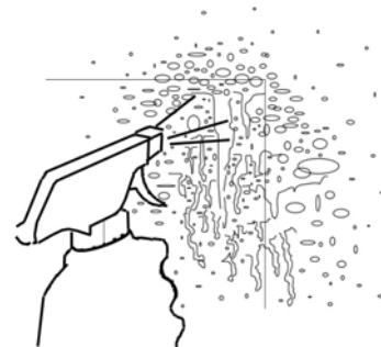
Beginning to spray top right corner of glass before putting film on it
